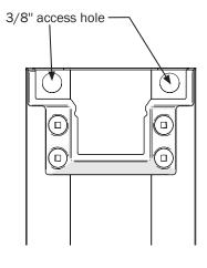
RECOMMENDED: use bracket as reference for location to drill. Mark center of channel before drilling.
