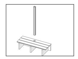
**Step 2:** Cut one 2" x (8" or 10") board to fit between joists. Place flush against post and bottom decking
