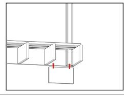
**Step 3:** Fasten cut board to joists on either end with three wood decking screws
