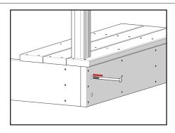
**Step 5:** Place the Strong-Tie Bracket over the top bolt, and fasten bolts using a standard washer followed by a nut.
