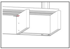
**Step 4:** Measure and mark holes for the Post Mount spaced at 5" on center. Use %6" drill bit with a shank at least 6" long. When measuring, ensure hole aligns with simpson strong tie. Keep power drill straight while drilling.
